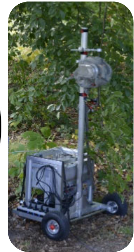
Portable MRI Formation of embolisms in fruit trees in the field
